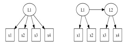
Figure 3.7: The structure on the left has three vanishing tetrad differences whereas the structure on the right only has one.
